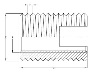
Female thread A = M16 Length B = 22 Male thread E = 20.0 Min hole depth blind hole = 27
